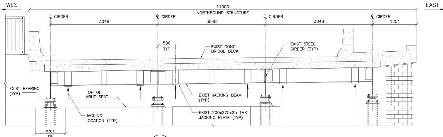
**2 NORTH ABUTMENT - FRONT ELEVATION**
